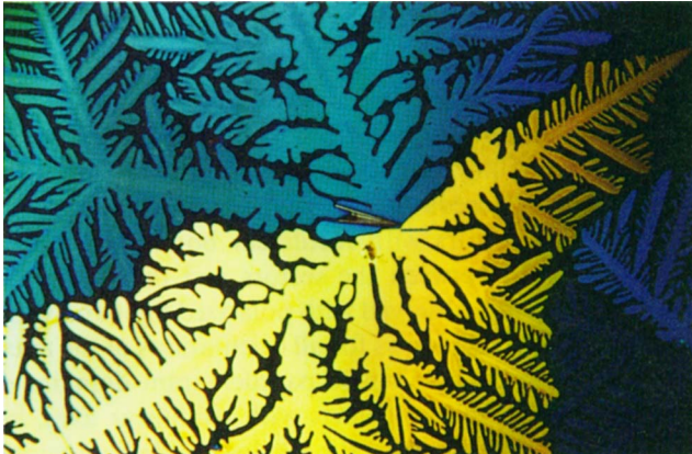
Plate 2. Mesophase of I.1 with digitized contours obtained by slow cooling of the liquid phase and viewed between crossed polarizers, with a wave plate inserted ( T = 152^{\circ}\text{C} ).
