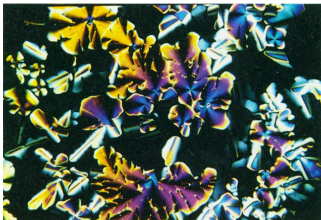
Plate 3. Mesophase of I.3 obtained by slow cooling of the liquid phase and viewed between crossed polarizers ( T = 239^{\circ}\text{C} ).
